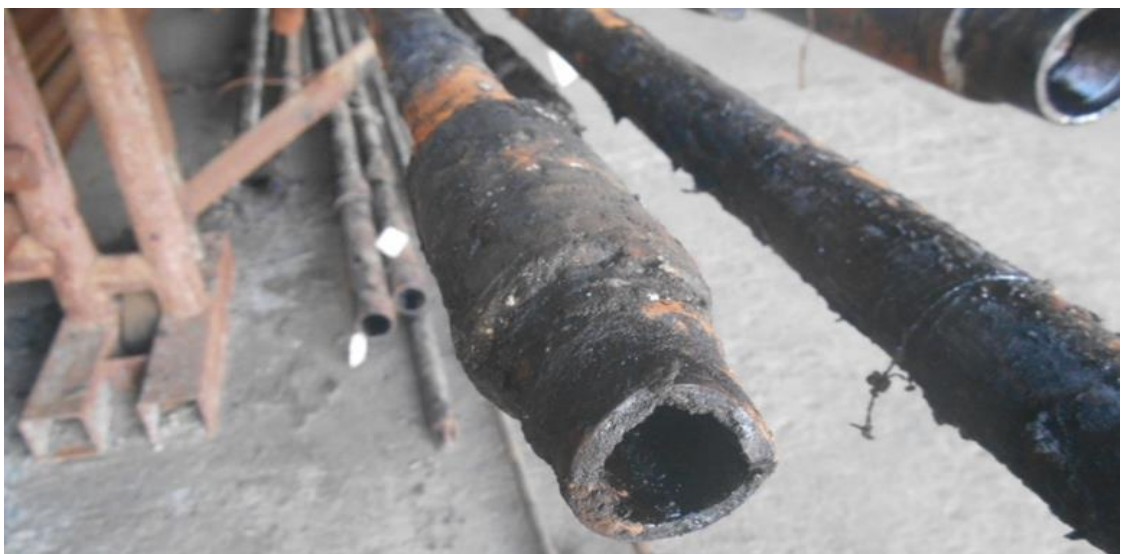
Figure 3 – Destruction of a sucker rod pump
