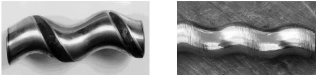
Figure 2 – Worn PCP rotors
