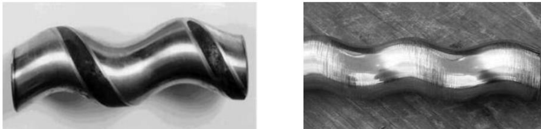
Figure 2 – Worn PCP rotors
