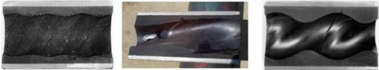
Figure 1 – Worn PCP elastomers and stators
